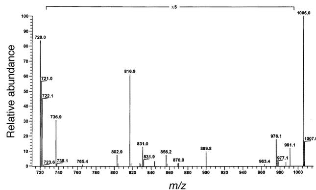
**Fig. 3** HPLC–APCI–MS/MS spectrum of the ion peak at  $m/z$  1006 obtained from peak 3 (collision energy at 50% of the scale)
