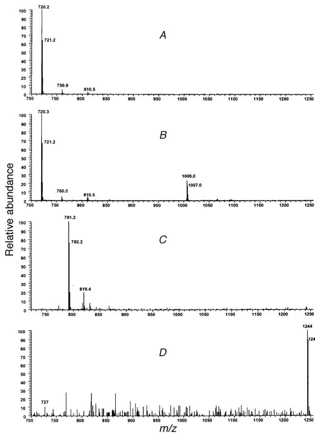
**Fig. 2** Mass spectra obtained from chromatograms (see Fig. 1 for chromatographic conditions). (A) APCI–MS spectrum of peak 1 (spectra of peaks 2, 4, 5, 6, 7 and  $C_{60}$ , not shown here, are identical with that of peak 1). (B) APCI–MS spectrum of peak 3. (C) ESI–MS spectrum of peak  $x_5$ . (D) ESI–MS spectrum of peak 7
